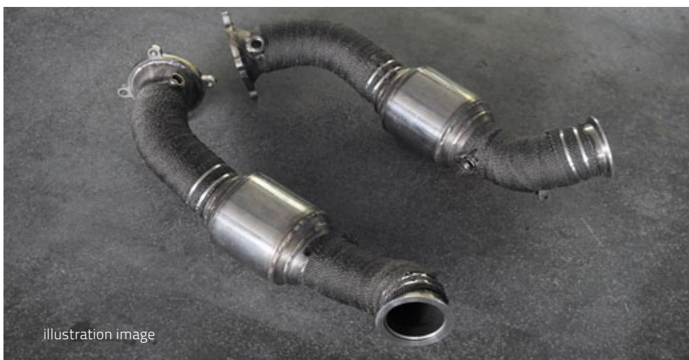
Down pipe with EUR6 with Cat 200 Cell
