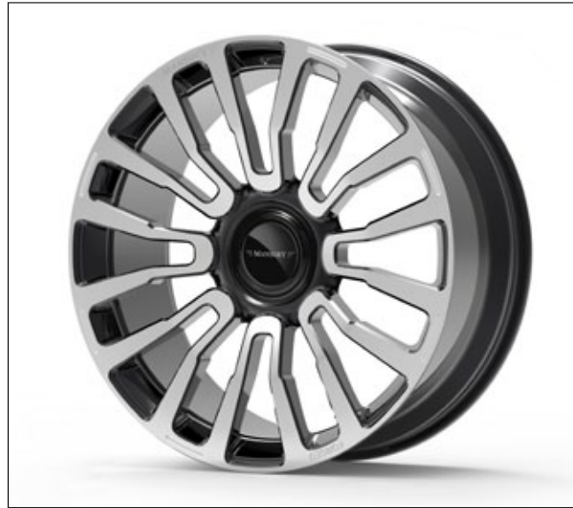
Y.8 wheel 24" fully forged wheel ..... Y8 24 10 25 112 B Diamond black 1pc., 10x24, ET25, 5x112 with wheel cap
