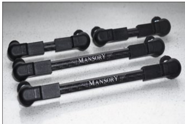
MANSORY Lowering Suspension ..... BBE 900 101 - 2 level adjusting rods front axle - 2 level adjusting rods rear axle Lowering of approx 20-30 mm
