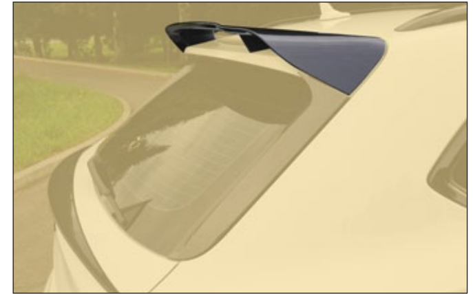
Roof spoiler BBE 630 771 with MANSORY logo - visible carbon visible carbon fibre glossy*
