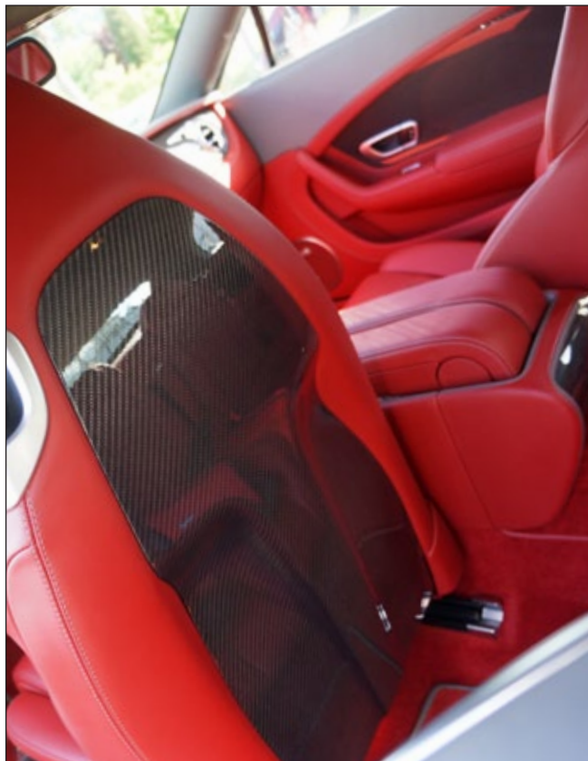
Carbon cover - seat rear panel ..... 505 393 751 ↻ modification only, OE-part required
