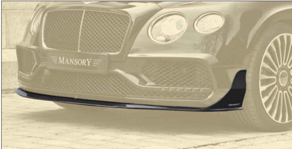
Race front splitter for MANSORY front bumper 2016 visible carbon fibre without clear coat
