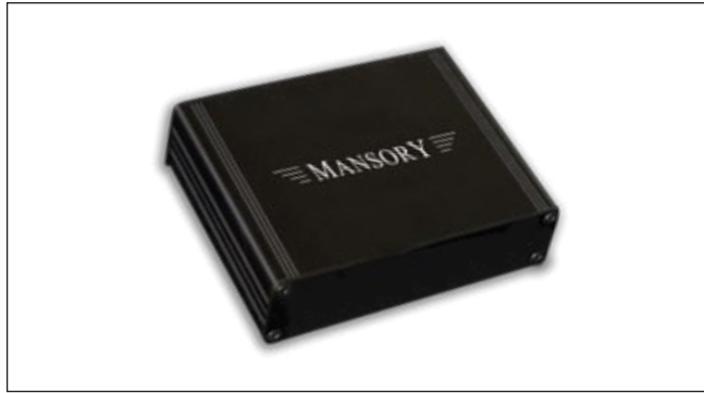
Electronic lowering module ..... BFS 250 050 The standard-lowering settings for Bentley are 30mm for the front axle and 20mm for the rear once. Fine adjustments of about +/- 20mm can be adjusted by manual turn screw operation. To keep the suspension comfort drive the module turns into original settings at a speed over 70 km/h by an automatic speed-control regulation. All moduls are TÜV certificated and come with a standard PAP adaptor.
