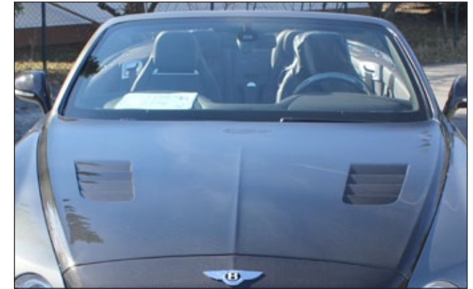
Engine bonnet ..... 505 110 001 visible carbon fibre without clear coat Primed engine bonnet ..... 505 110 002 not visible carbon fibre with visible carbon fibre without clear coat air outtakes
