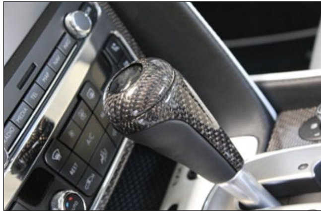
Gearshift lever 505 363 011 designed gear shift lever visible carbon fibre without clear coat
