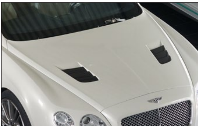
Engine bonnet, primed ..... 505 110 002 bonnet - not visible carbon fibre primed air outtakes - visible carbon fibre without clear coat
