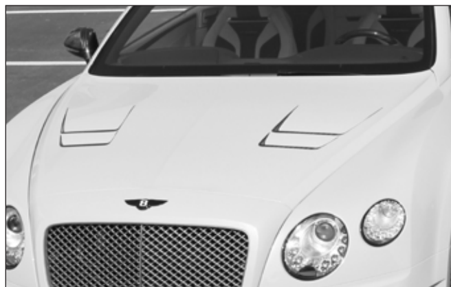
NEW engine bonnet, primed ..... 505 110 012 bonnet - not visible carbon fibre primed air outtakes contour - visible carbon fibre without clear coat
