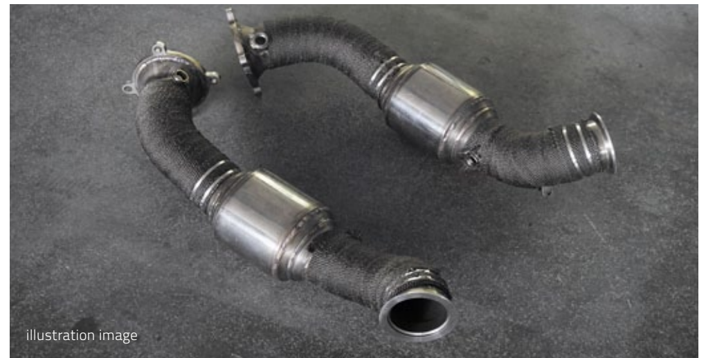
Down pipe with EUR6 with Cat 200 Cell - V8
