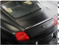
Complete trunk lid hatch with integrated rear spoiler,
