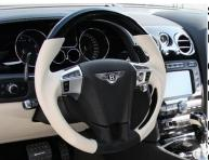
Sport steering wheel, Model: GT SPEED Diameter 385 mm
