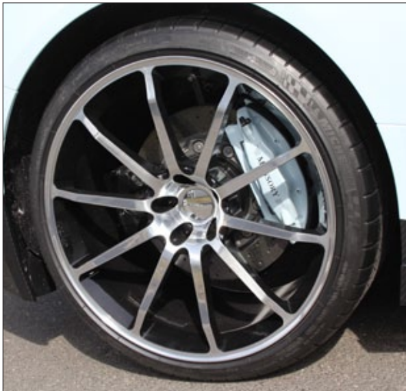
V.10 Fully Forged light-alloy wheels
