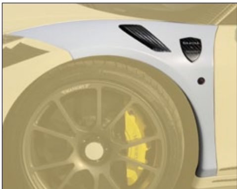
Front fender with air outtake ..... 458 000 94 visible carbon fibre primed without clear coat 2 parts set - left & right
