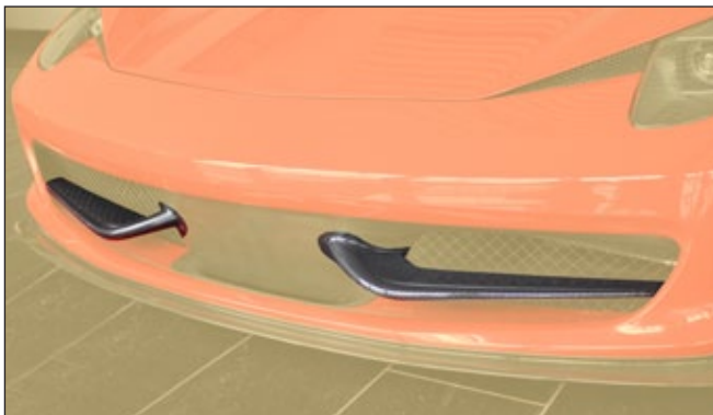
Air intakes Add-on ..... 458 102 871 visible carbon fibre primed without clear coat 2 parts set - left & right ⓘ not compatible with MANSORY Front kit (458 001 01)
