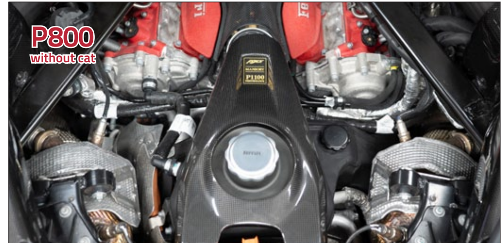
P800 without cat Performance software + Downpipe without Cat MPU FPM 80W Software upgrade 800 PS / 950 Nm, Flap controlled Mansory Exhaust System, Mansory High Performance Turbocharger Upgrade, Sports Air Filter, Downpipe without cat (C) modification only, OE - ECU required
