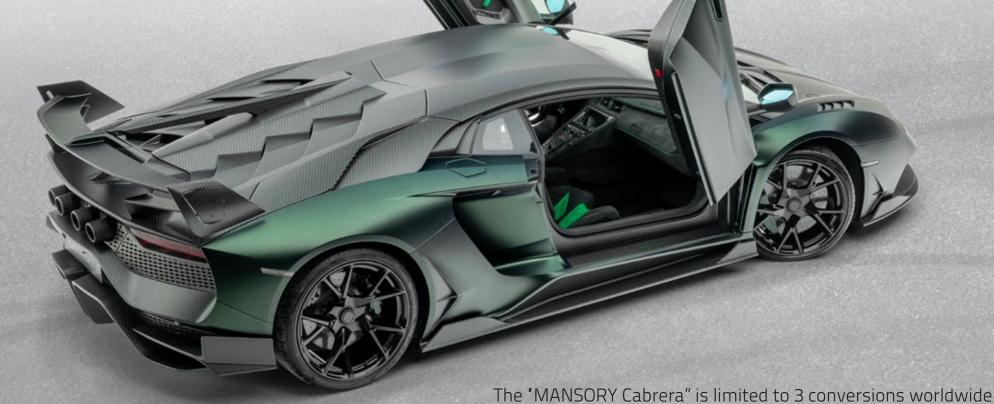
For example, the striking air inlets of the front apron optimise the fresh air flow of the radiator. Together with the specially developed front design, this also results in improved downforce for more road grip overall. At the sides, striking side skirts and the grown wheel arches show the well-known MANSORY signature. And here too, visual enjoyment and technical functionality go hand in hand. E.g. the new carbon components not only look impressively good, they also act as air fins
