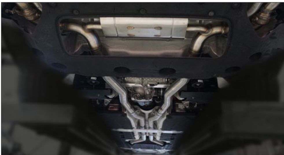
Sport Exhaust Muffler for MANSORY Rear diffuser LRR 222 219
