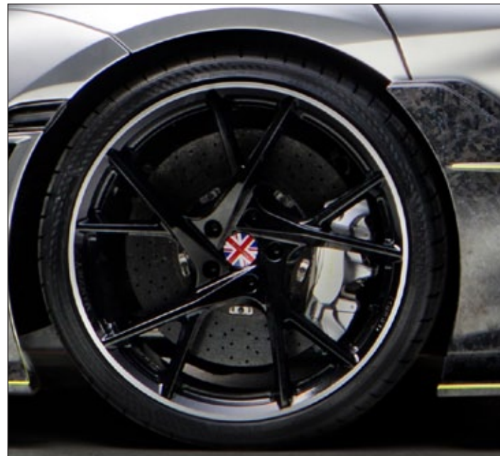
YN.5 Wheels ultra-light forged wheels FA: 9.5 x 20 inch YN5 20 95 34 112 R RA: 11.0 x 21 inch YN5 21 11 14 112 R
