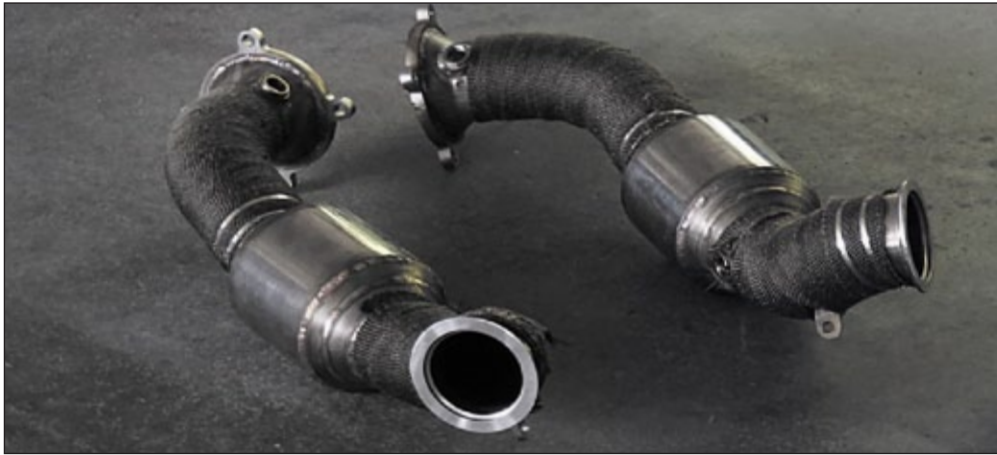
Down pipes with cat 200 cell
