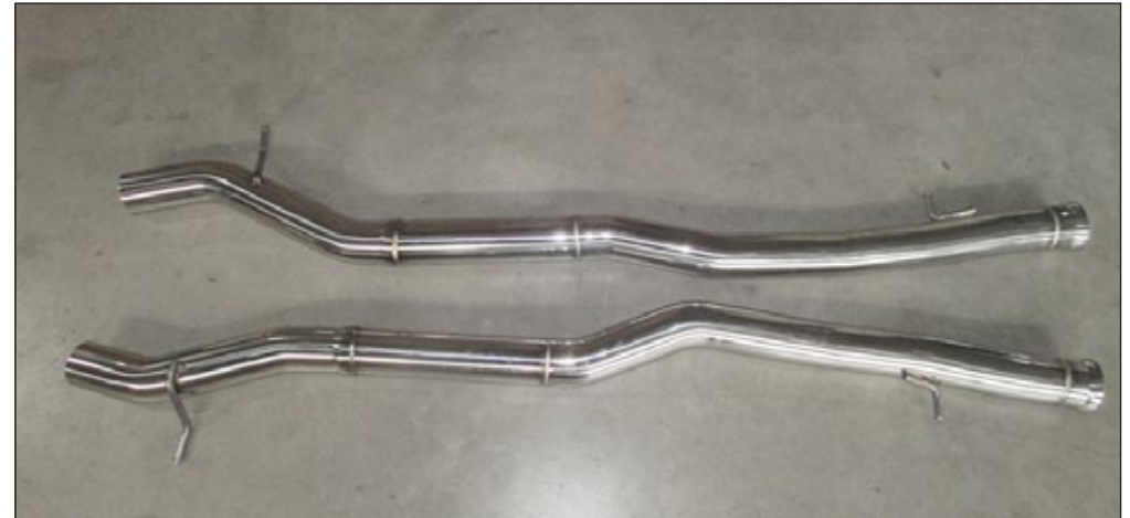
Exhaust middle pipes
