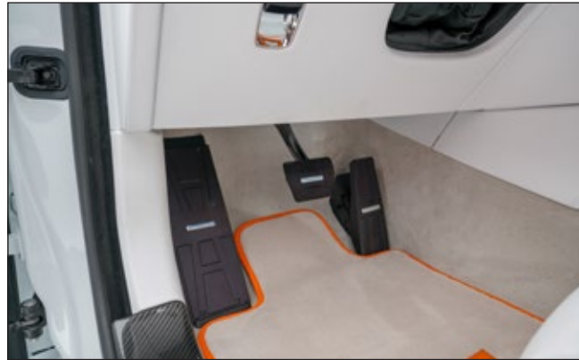
Sport pedals RNG 367 127 3 parts, acceleration, brake, foot rest
