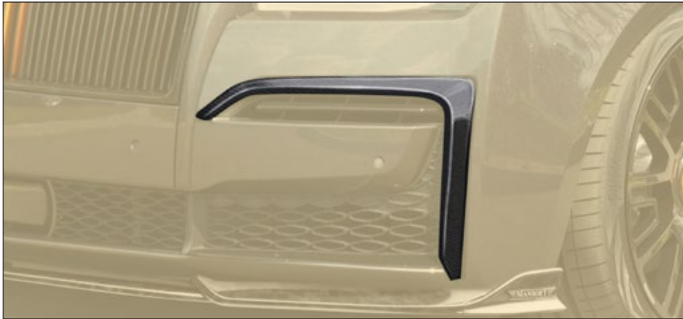
Front splitter visible carbon fibre glossy* 2 parts set - left & right
